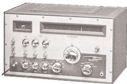
Heathkit HX10 Marauder 180WCW, AM, SSB, FSK 38kg 495x292x406mm
