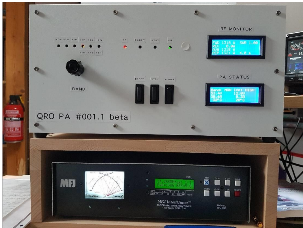
BETA, thermal test 1.3kW+ continuous
